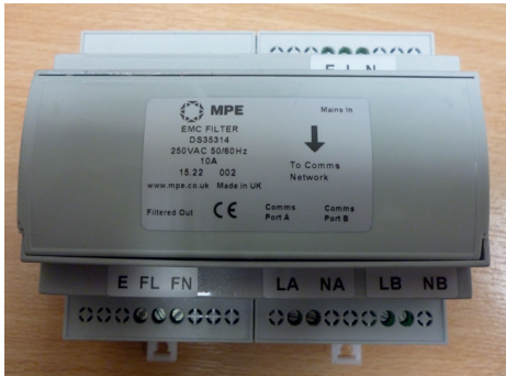
The custom EMC filter developed by MPE for TerOpta's TeroLight intelligent lighting system
