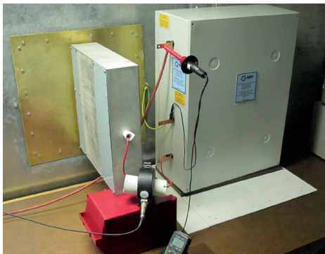
The new Marx pulse generator installed within MPE's in-house screened room test facility
