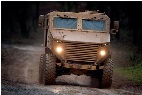
The 7.5t, mine-protected Foxhound features a V-shaped hull, which provides maximum protection to the crew. The hull, running the entire length of the vehicle, also includes the driveline, main fuel tank, generator, batteries and power pack. The Foxhound affords better flexibility and protection against IEDs, mines and roadside bombs than other light patrol vehicles and so replaced the British Army's Snatch Land Rover in the theatre of war in Afghanistan.
